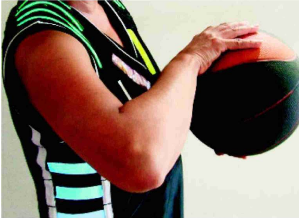
Electricity-carrying cotton thread weaves through the shirt from the computer.
