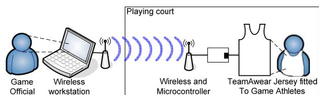
**Figure 1: Diagram showing TeamAwear during use**
